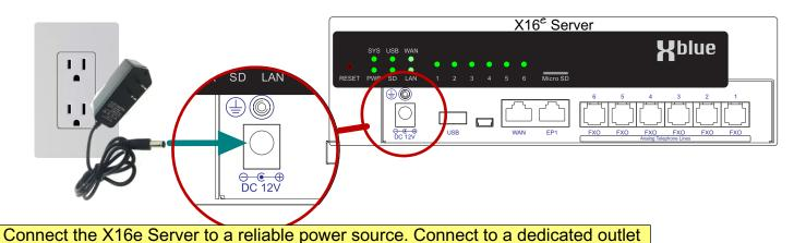
We recommend a battery-backed Uninterruptable Power Supply [UPS]
